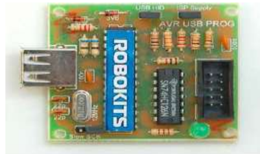
Figure(3.4). View of ISP connector
