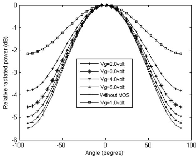
Fig. 10 E-plane radiation pattern of MOS loaded circular microstrip antenna with airgap ( $H_a = 1.0$  mm)
