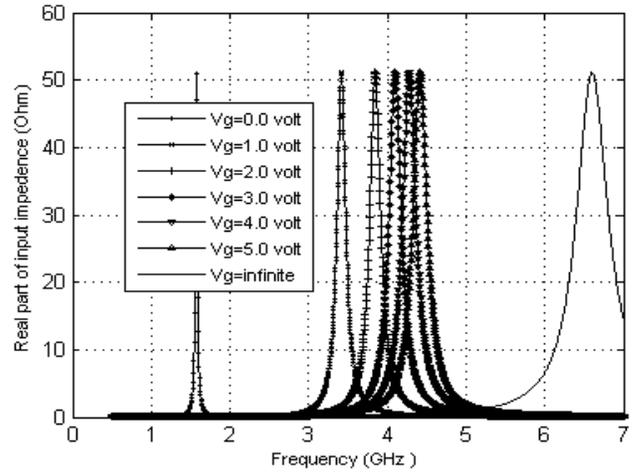
Fig.8 V ariation of input impedance with frequency with different bias voltage ( $V_g$ ) of MOS loaded circular microstrip antenna with airgap ( $H_a = 1.0$  mm)
