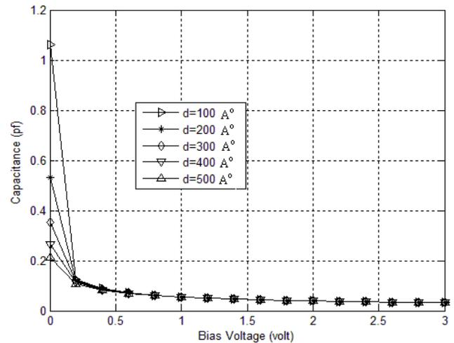
Fig.5 Variation of capacitance of a MOS with bias voltage
