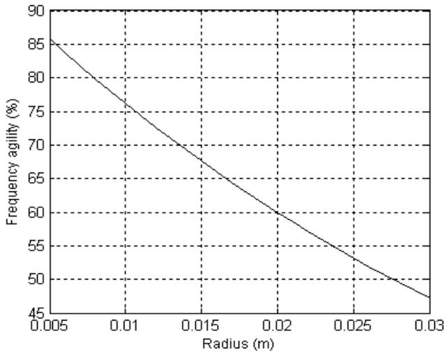
Fig.7 V ariation of frequency agility with radius of patch of MOS loaded circular microstrip antenna with airgap ( $H_a = 1.0$  mm)
