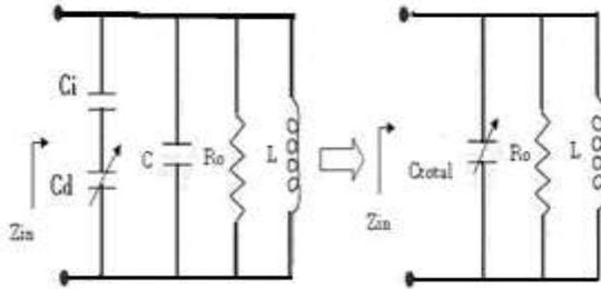
Fig.3 Equivalent circuit of MOS loaded circular microstrip antenna
