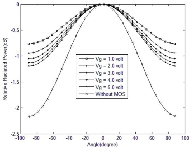
Figure 11: H-plane radiation pattern of MOS loaded circular microstrip antenna with airgap ( $H_a = 1.0$  mm)
