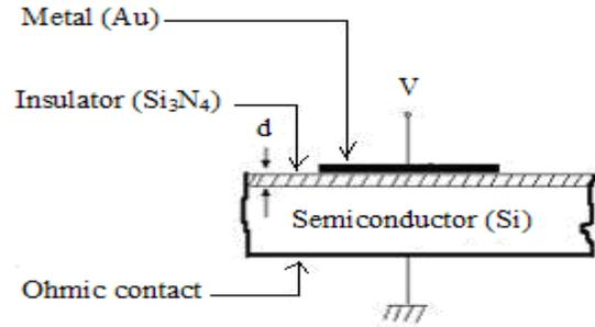
Fig. 2 Schematic of MOS capacitor
