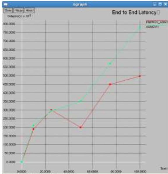
Fig 8. Comparison of end to end delay for AOMDV and ENERGY_AOMDV using 60 nodes
