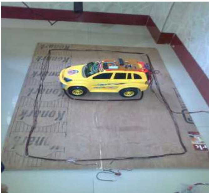
Figure7. Photograph of Tx Coil (plywood) and Rx Coil (Bottom of the vehicle) inside the magnetic field region
