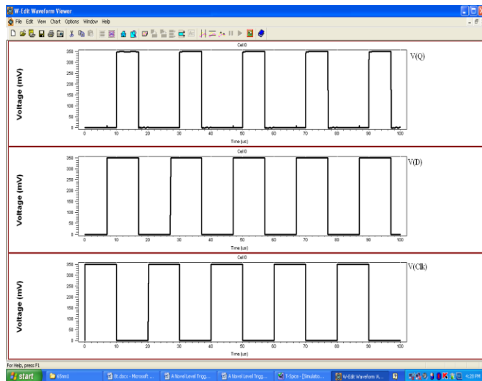
Figure 3. Input Output waveform of proposed 8t latch
