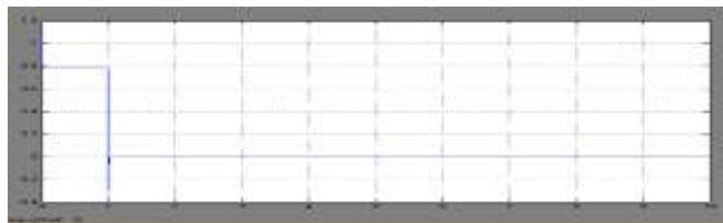
Figure 15. Impulse response of the model of fuel cell system in closed loop configuration with minimum order observer.
