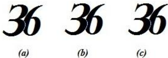
Figure 8: Selective attention . (a) An input pattern. (b) The recognizer gradually reinforces pixels that corresponds to objects in its template library, and inhibits those that do not, yielding a partial recognition. (c) After a delay, attention is switched to unmatched regions, and another match to the library is found (after Fukushima).
