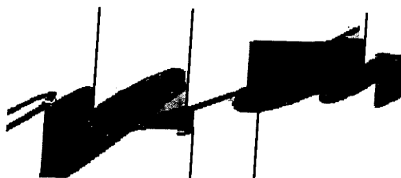
Figure 6: Dissection based on search and deflect. The initial path of the cut trajectory is along a column corresponding to a minimum in the upper profile of the image. When black is encountered the path is modified recursively, seeking better positions at which to enforce a cut. In this way, multiple cuts can be made at positions which are in the shadow region of the image.
