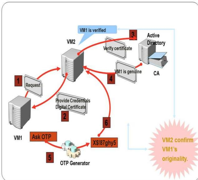
Figure 5 Securing Communication between Virtual Machines
