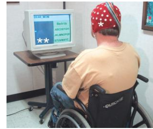
Figure 4. Example of an EEG-based BCI platform. Notable elements include the electrode cap worn (asterisk) by the subject and the viewer screen (double asterisks) for which the subject controls the cursor on the screen (BCI computer not shown) by various EEG signals and signal processing methods (i.e., sensorimotor rhythms, SCP, or P300 paradigm)
