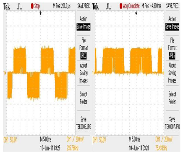
Figure 10. Output line volt and volt across switch for simple boost control
