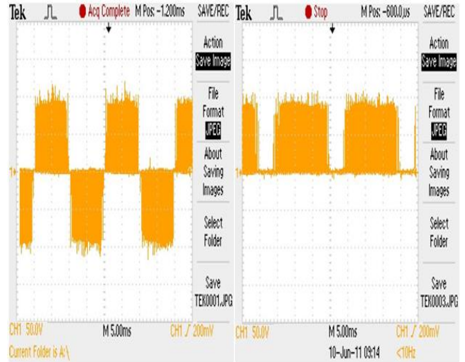
Figure 12. Output line voltage and voltage across switch for maximum constant boost
