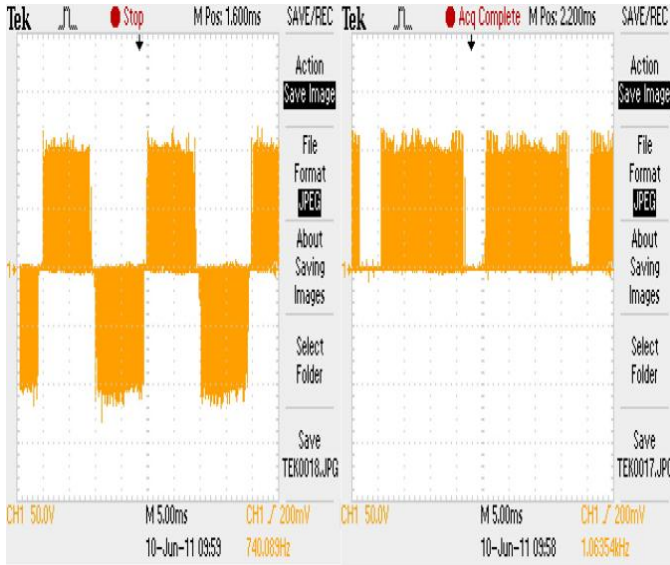
Figure 11. Output line voltage and voltage across switch for maximum boost control
