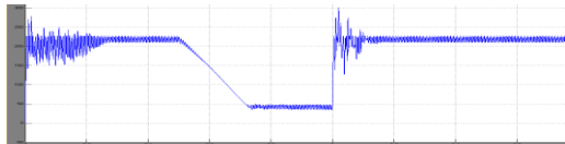
Figure.2 DC link capacitor voltage of normal rectifier.
