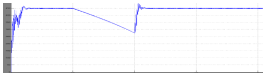
Figure.3 DC link capacitor voltage of Vienna rectifier.
