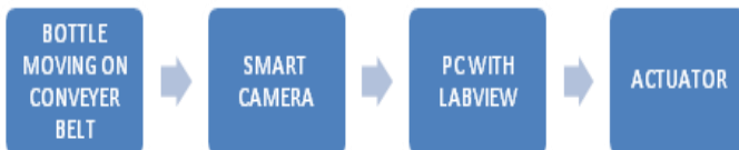
Fig 3. Block diagram of the proposed technique
