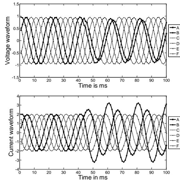
corresponding phase which are involved in the fault (A & B) increases and voltage decreases as shown in Fig. 5.
